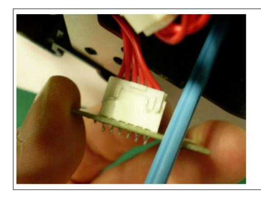
(5) Take out the OEM chip and install compatible new chip.
