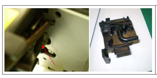
(2) Then disconnect the tube of the PIPE, and remove the sliding door.
