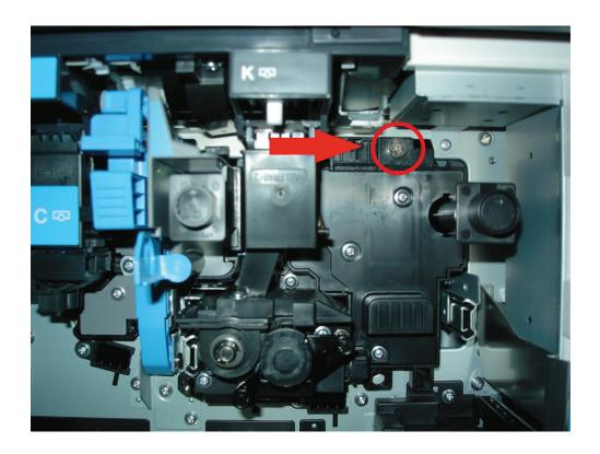
10.Close the front cover, wait until machine recognizes our new chip, will reset the full lifecycle and will make an stabilization process as a new drum unit installed.
