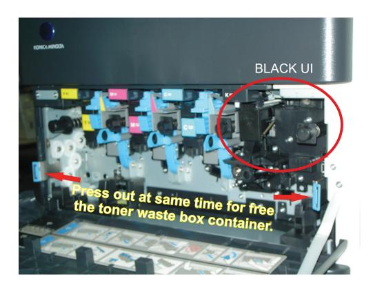
2 . Looking at the front,unscrew the big screw, see at the following photo for locate it. Not possible to fall, it is just for ensure the UI is not moving anymore inside the machine.
