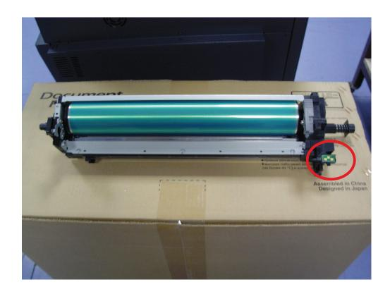
8. Job done. Now we need to install again the drum unit over the developer unit, reverse action from step 5.
