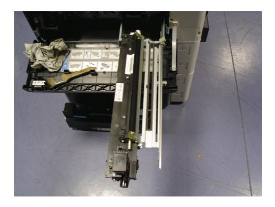
7. Locate the chip on the drum unit and replace for our new chip.
