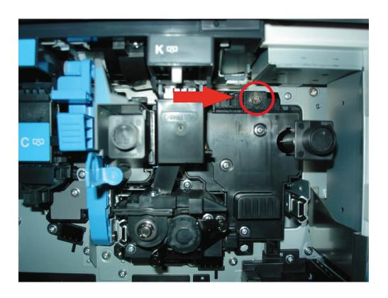
3. Next step is slide the image unit out by the holder, till the end.
