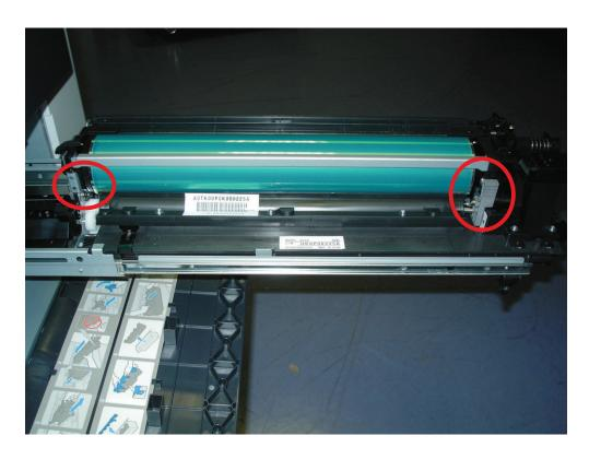
6. Once drum unit is out only developer unit will be hanged on the rails, as the photo.
