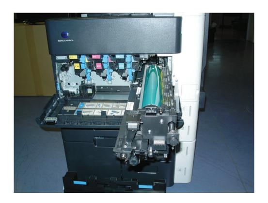
5. Now we have to separate the drum unit from the developing unit, it is easy to do but please be very carefull not to damage the opc surface of the drum ( suggested action to cover it ). Look it on the direction of the photo and with the two hands at same time take out the drum while pressing with your fingers. Note that drum unit is not leaved, just lift it.
