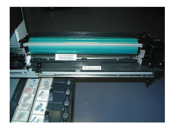
9. Ensure that it is properly fit, and push inside the machine again the black image unit till the end, then you can screw again it to the machine and then reinstall the waste toner box back by pressing inside strong until it get armed for end our work.
