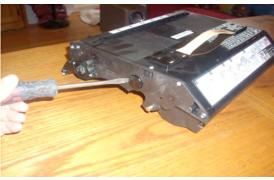
Step 4 - Locate chip on side of unit and using a small flat screwdriver gently pry out the small round plastic housing of the chip. Note: Make sure the whole housing comes out. Often it comes apart and leaves the legs still inside the drum. You know this when the new chip will not fit in.
