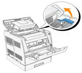
**Step 2** - To remove the used drum cartridge, push up the lever on the right side of the printer.
