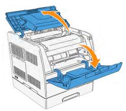
**Step 1** – To open both covers on the printer, grab the notch in the front door and pull forward. Lift the top cover and push back.
