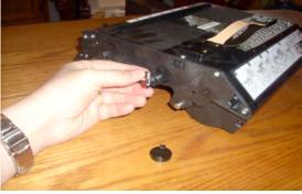
**Step 5** - Gently place new chip into photoconductor unit. Note: pay attention to location of chip legs and gently push into place.
