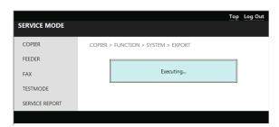
4. Check that a setting information file (service.dcm) exists in the directory directly under the root of the USB flash drive.
