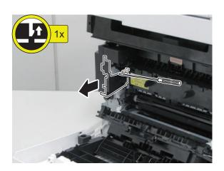
2. Free the harness from the guides, and disconnect the connectors.
