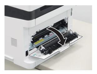
2. Remove the Secondary Transfer Roller.
