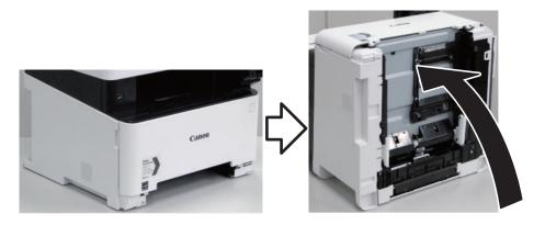
2. Remove white Separation Roller Guide, then remove the Separation Roller while disengaging the claw.
