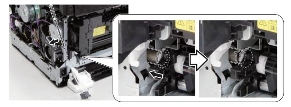
4. With the Cartridge Cover opened, remove the screws, and pull out the ITB Unit while lifting the stoppers and holding the handles on the left and right sides.
