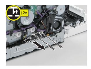
2. Free the harness, and remove the Fan Unit.
