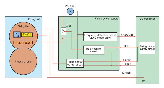
The DC Controller monitors the fixing temperature detection signal and outputs a fixing control signal according to the detected temperature. The fixing control circuit controls the Fixing Heater on the basis of this signal, and controls the temperature of the Fixing Heater to the target value.
