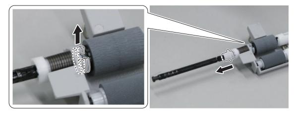
2. Move the Roller Shaft, and remove the Parallel Pin.
