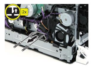
2. With the Cartridge Cover closed, rotate the lever approximately 45 degrees in the direction of the arrow while pulling it toward the front, and then pull it further toward the front.
