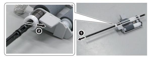
3. Turn the Roller Shaft in the direction of the arrow, and remove it after aligning the protrusion with the hole on the Roller Holder.
