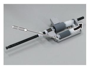
2. Remove the ADF Pickup Roller.
