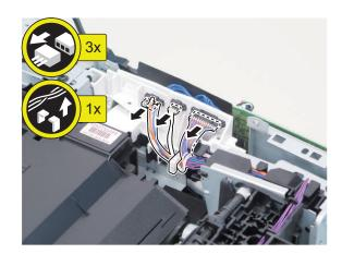
4. Remove the Fixing Assembly.
