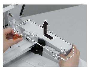
5. Remove the screws, and remove the ADF Pickup Feed Unit.
