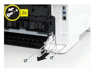
2. Remove the Shaft Retainer Holder.
