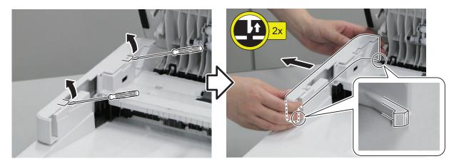
4. Release the boss, and remove the ADF Rear Cover in the direction of the arrow.
