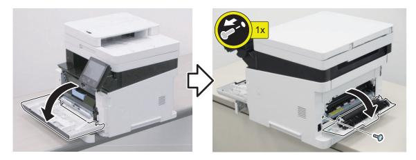
4. Release the claws while opening the Right Cover in the direction of the arrow.
