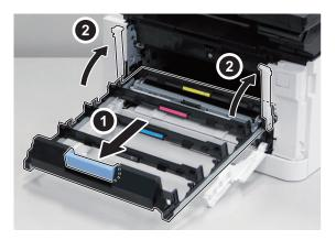
2. Remove the pin from the groove of the left side rail while lifting up the left side of the Cartridge Tray, and turn the Cartridge Tray counterclockwise to remove the tray.
