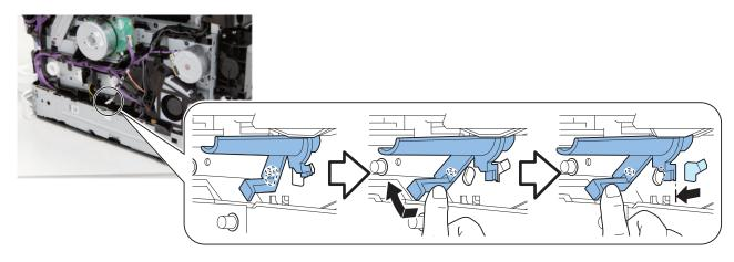
4. Slide the gear to the left to disengage the shaft from the ITB Unit.
