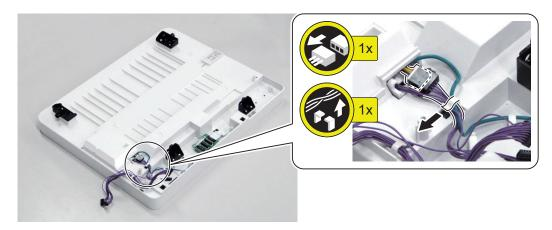
2. Turn it over so that the front side is facing up, and remove the Sensor Mounting Base.
