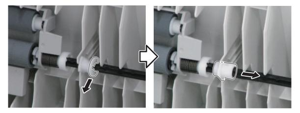
4. Remove the E-ring and the bushing, and remove the ADF Roller Unit.
