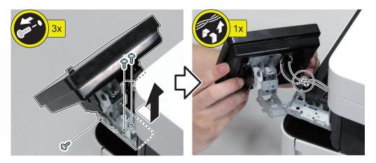
6. Remove the Panel Rear Lower Cover. Disconnect the connector and HDMI Cable, and free the harness from the Wire Saddle.
