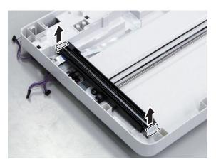
2. Remove the Flat Cable, and remove the Reader CIS Mounting Base from the Timing Belt.
