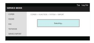
**5.** Restart the host machine, enter service mode, and confirm that the setting information is reflected. This completes the procedure for importing a setting information file.
