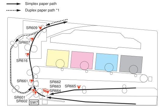
Occurrence of a jam is judged by whether paper is in the sensor area at the timings stored in the DC Controller. When the DC Controller judges that a jam has occurred, the printing operation is stopped and the jam is notified to the Main Controller at the same time.
