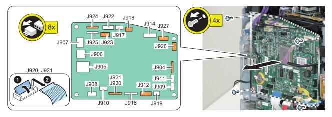
2. Actions after replacement: "After Replacing the Main Controller PCB" on page 169
