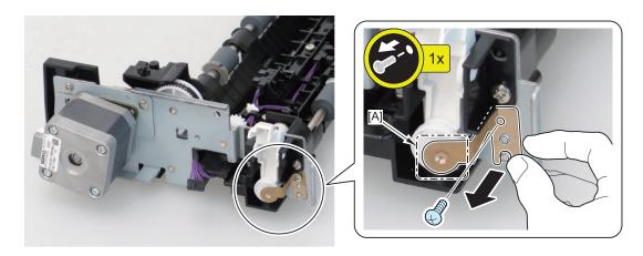
2. Remove the Pressure Release Lever.
