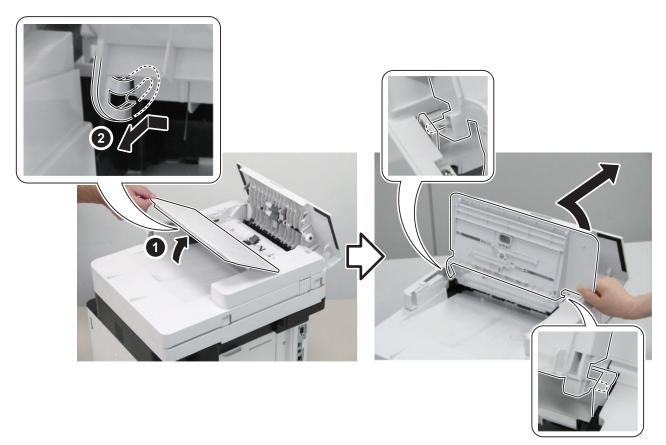
3. Release the hooks, and remove the ADF Front Cover in the direction of the arrow.
