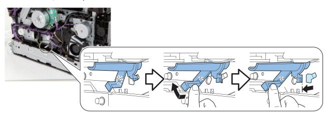
3. Slide the gear to the left to disengage the shaft from the ITB Unit.
