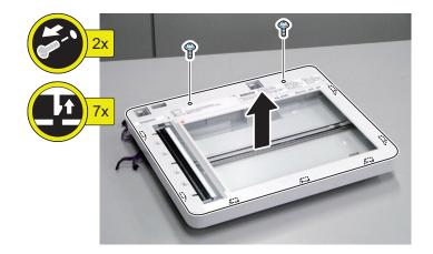
2. Actions after replacement: "After Replacing the Reader Upper Cover Unit" on page 182
