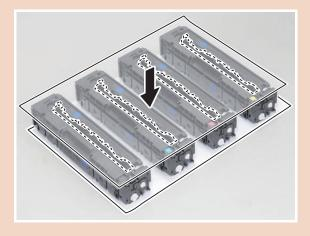
1. Pull out the Cartridge Tray, and remove the Toner Cartridges (Y, M, C, and Bk).
