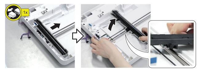
3. Lift up the Reader CIS, and remove it in the direction of the arrow. Be careful not to lose the springs.
