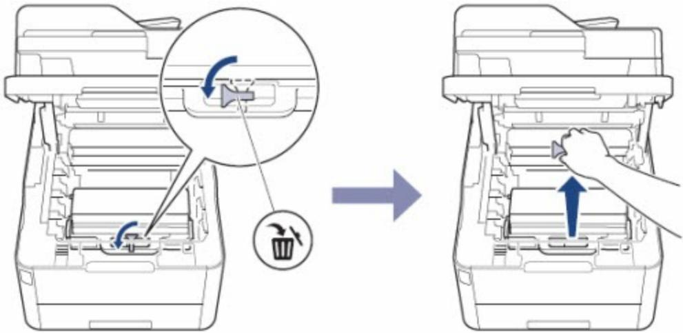
6. Hold the green handle of the waste toner box and remove the waste toner box from the machine.
