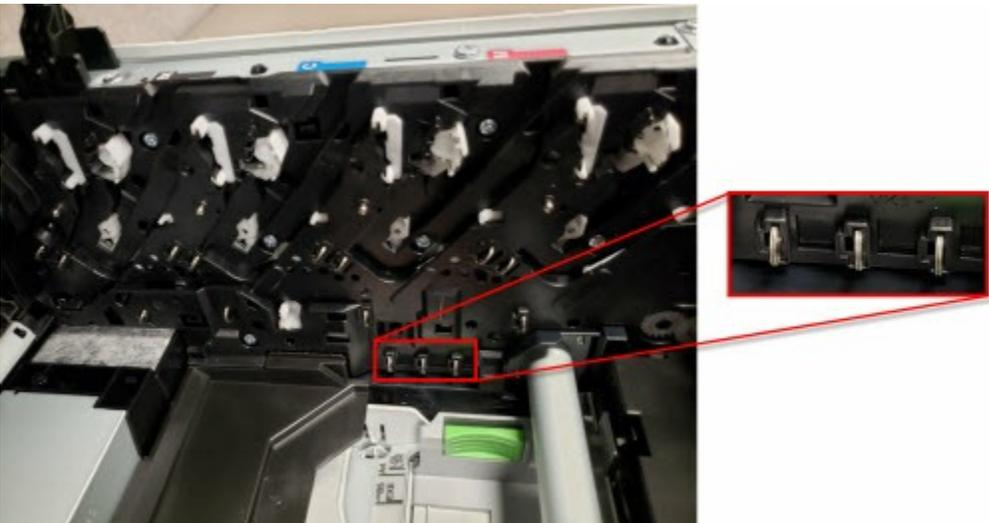
10. Push in on each of the three metal contacts inside the machine to make sure each one springs back into place.
