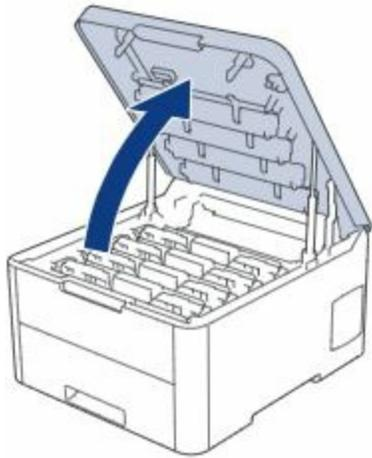
3. Remove all of the drum unit and toner cartridge assemblies.
