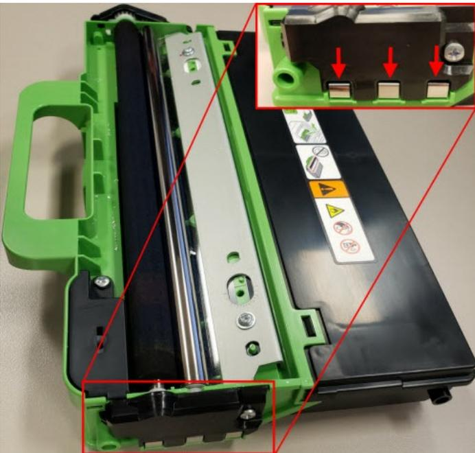
9. Use a dry lint free cloth to clean the three corresponding metal contacts on the right hand side inside the machine. These look like small key rings.
