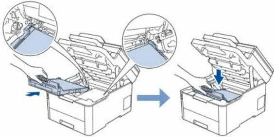
13. Reinstall the drum unit and toner cartridge assemblies into the machine by sliding them into the correct slot by
