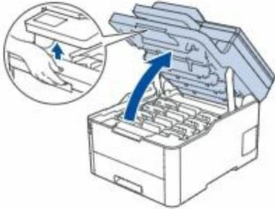
3. Remove all of the drum unit and toner cartridge assemblies.
