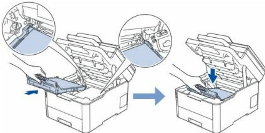
13. Reinstall the drum unit and toner cartridge assemblies into the machine by sliding them into the correct slot by matching the toner cartridge color to the same color label on the machine.
