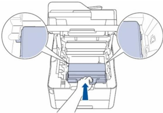
12. Install the belt unit back into the machine. Make sure the belt unit is level and fits firmly into place.
