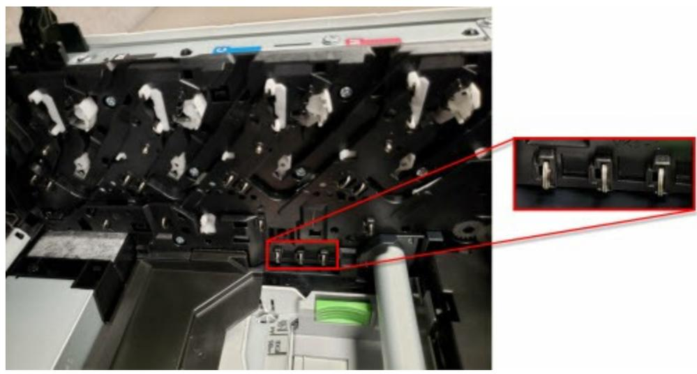
10. Push in on each of the three metal contacts inside the machine to make sure each one springs back into place.
