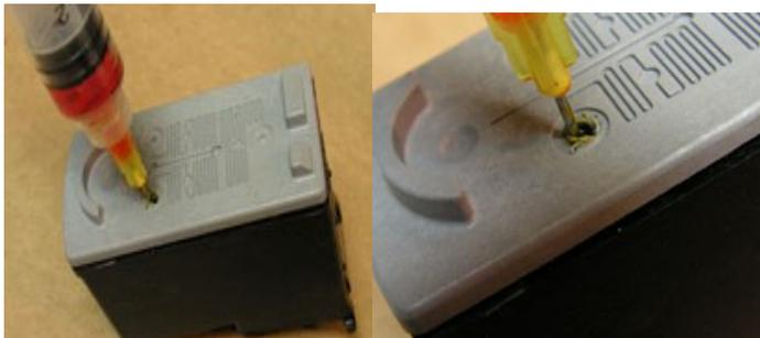
Insert needle into vent hole down into cartridge sponge material. Do not insert all the way into the cartridge. Note on the image to the left that there is adequate room for air to get out of the cartridge on the side of the needle. Slowly inject ink into cartridge. The slower the better.
