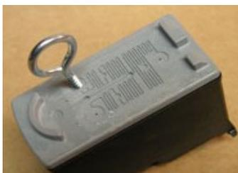
4. Take twist tool (eyelet screw, drill bit) and enlarge the cartridge vent holes. Or you can use the drill and the drill bit, just make sure that the drill bit just a little bigger than needle. The eyelet screw which we include with our kits is an excellent size for a 20g blunt needle
