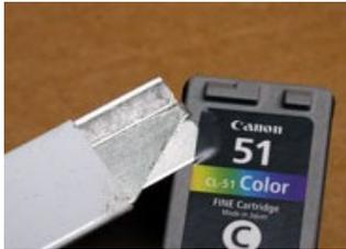
2. Remove top label. The easiest way to remove the top label is to take a box cutter or similar style razor (Exact as an example) and wedge underneath label to raise the top corner
