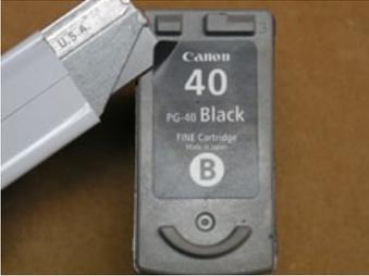
2. Remove top label. Take a box cutter or similar style razor (Exact as an example) and wedge underneath label to raise the top corner.
