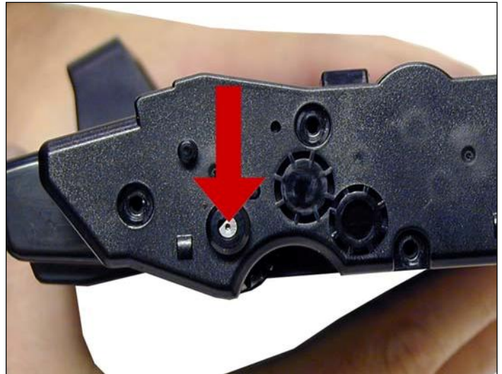
33. Take the right side end cap align the drum axle keyed end so it will fit into the keyed slot of the end cap. Snap the end cap into place.
