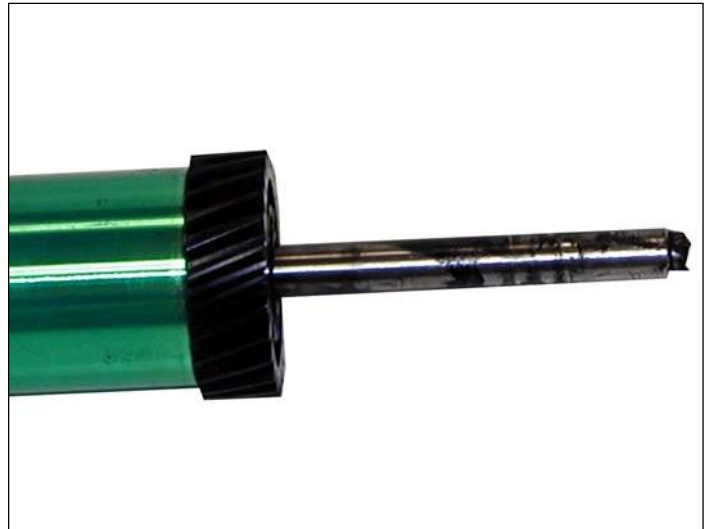
16. The gear side of the drum axle shaft has conductive grease on it. Regardless of if you are replacing the drum or not, clean the old grease off, and replace with new.
