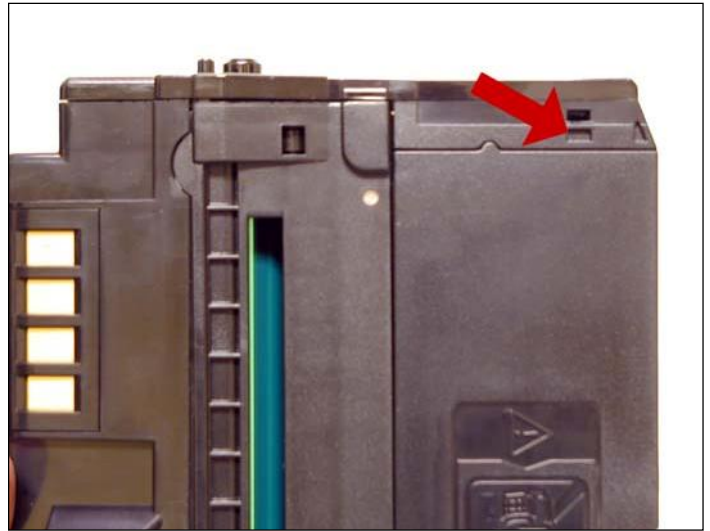
4. Press in on these tabs, and remove the end cap.
