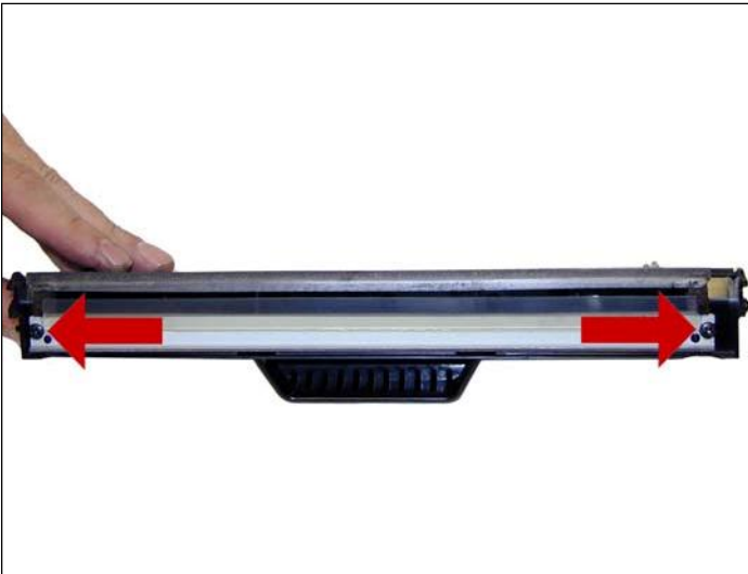
15. Install the cleaned or new doctor blade and two screws.
