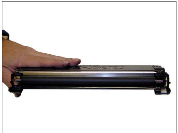
27. Clean the developer roller with a dedicated DVR cleaner, and replace into the hopper. Install the gear side first.
