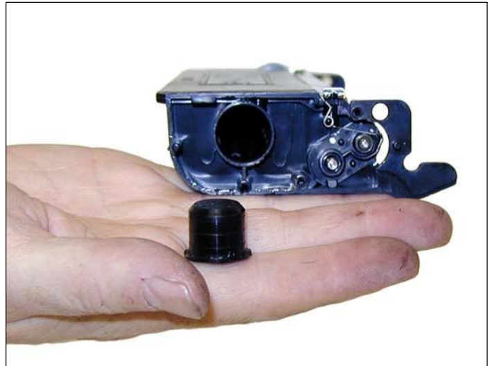
18. Carefully pry out the fill plug on the toner hopper, and dump out any remaining toner. The fill plug can be difficult to remove. Take a small common screwdriver and work it around the edge lifting slightly until it comes loose.
