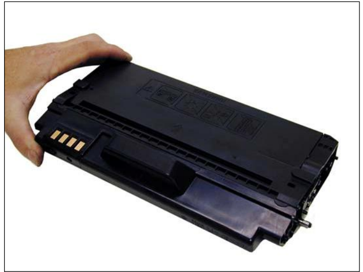
32. Slide the middle top cover/PCR assembly into place. Make sure the two middle tabs fit under the edge of the waste hopper.
