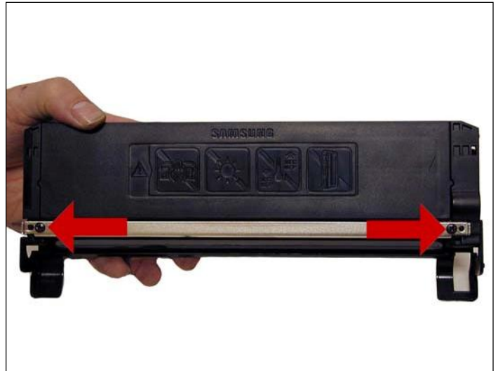
23. Remove the 2 screws from the doctor blade, remove the blade.
