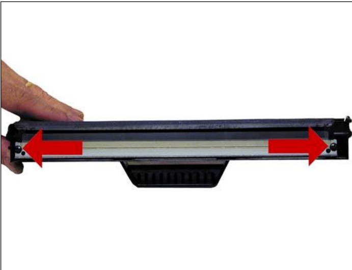
13. Remove the two screws from the doctor blade, remove the blade.
