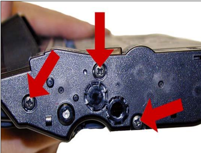
34. Install the three screws into the end cap.
