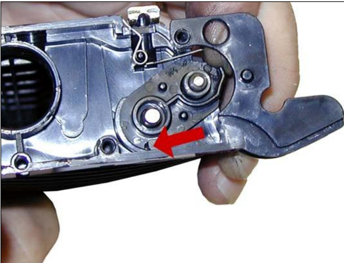
21. Press in on the bushing tab, and remove the bushing. Be careful not to lose the spring.
