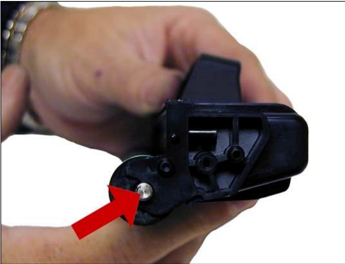
12. Remove the drum axle from the clips on both sides of the waste assembly. Remove the drum.
