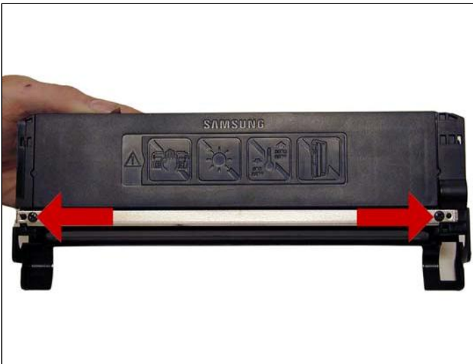
26. Install the doctor blade and two screws.
