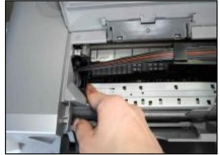
Adjust the tube length and move from Left to right for several times.
