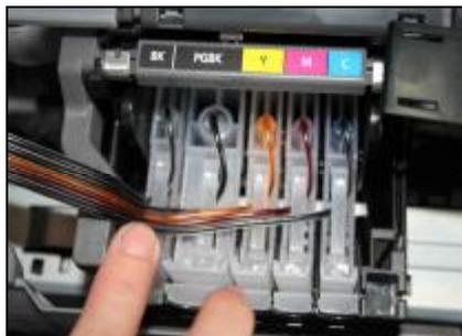
Then put the CISS cartridges into printer
