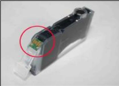
Carefully remove the original chips
