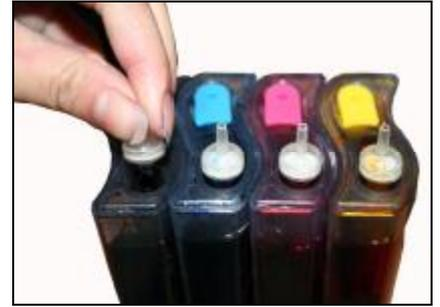
Put the Air-filter into the Air-hole
