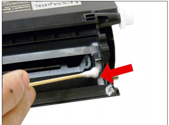
13. Clean the white developer roller seals with a cotton swab.
