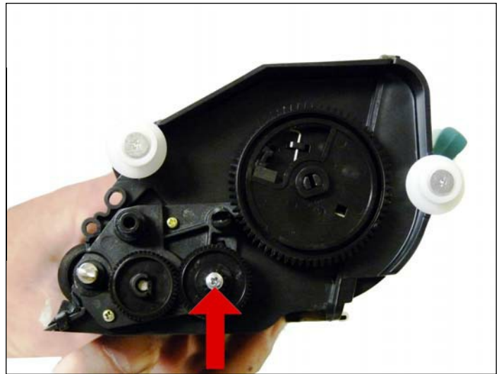
9. Remove the screw and lower idler gear.
