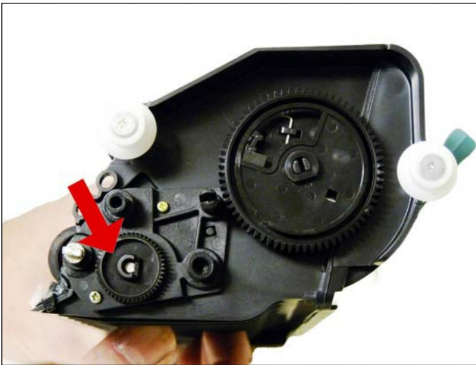
10. Remove the feed roller gear.
