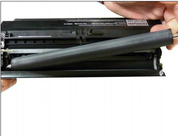
12. Remove the developer roller.
