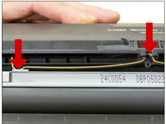
18. Install the doctor blade making sure it is positioned correctly and install the leaf spring.
