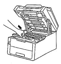
4. Hold the green handle of the belt unit and lift the belt unit up, then pull it out.
