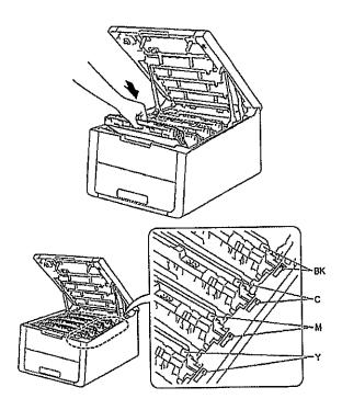
7. Close the top cover of the machine. You will hear a loud click when the top cover is closed firmly.
