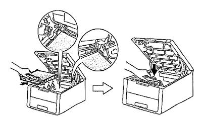
6. Reinstall the drum unit and toner cartridge assemblies into the machine by sliding them into the correct slot by matching the toner cartridge color to the same color label on the machine.
