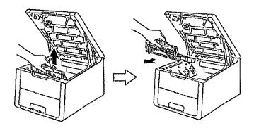
5. Unpack the new belt unit and put the new belt unit in the printer.
