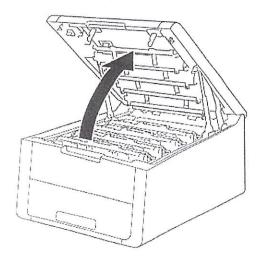
**IMPORTANT:** The top cover must ALWAYS be completely open when removing or installing consumables. Failure to completely open the top cover may cause damage to the machine.
