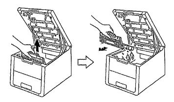
5. Unpack the new belt unit and put the new belt unit in the printer.
