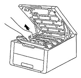
4. Hold the green handle of the belt unit and lift the belt unit up, then pull it out.
