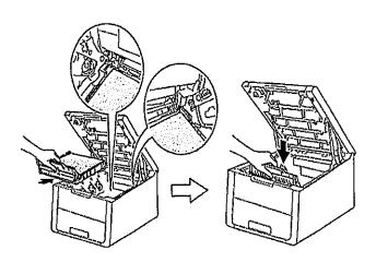
6. Reinstall the drum unit and toner cartridge assemblies into the machine by sliding them into the correct slot by matching the toner cartridge color to the same color label on the machine.
