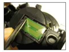
Replacing Chip - Remove 4 sides
