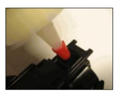
2. Shake the toner powder well until it appears liquid like. Open cap carefully and screw on the funnel. Refill the the toner....apply plug, then clean any spilled toner thoroughly by using a vacuum.
