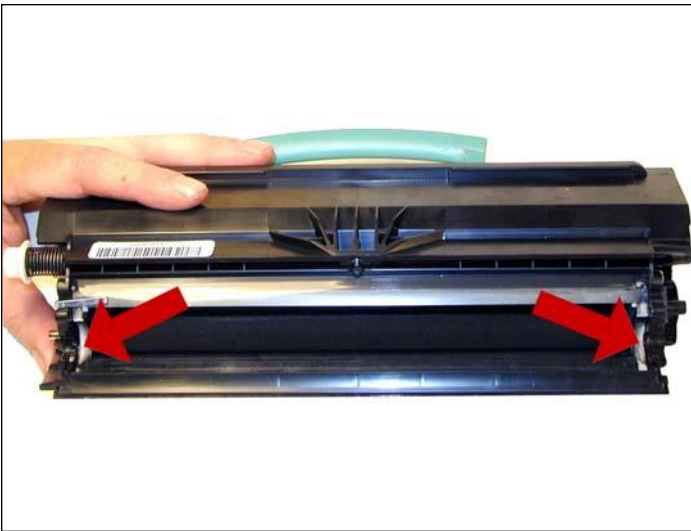
8. Clean the white developer roller seals with a cotton swab.
