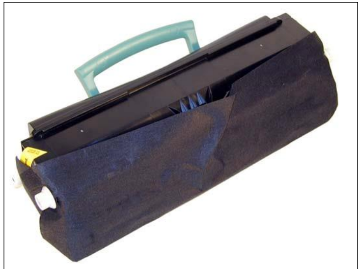
17. If the felt cover is available, wrap the cartridge as indicated. This cover helps protect the developer roller from damage.
