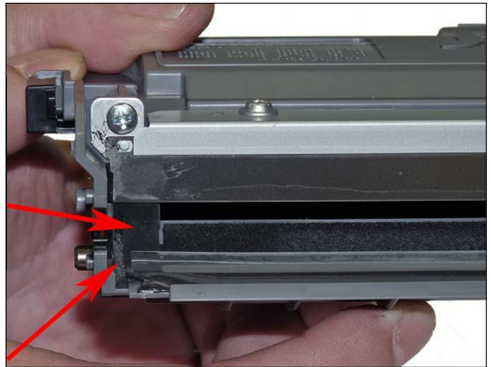
10. Vacuum the doctor blade clean. Until new blades are available, we do not recommend that the doctor blade be removed or the developer roller felt seals disturbed. The doctor blade can be easily cleaned by blowing the excess toner off, and wiping it down with a lint-free cloth. Be very careful not to leave any lint behind!
